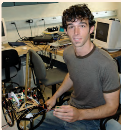
Gabe Graham working on a two-dimensional inverted pendulum stabilized by moment exchange wheels.
