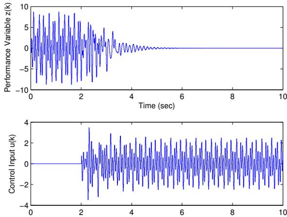
Fig. 3. Closed-loop disturbance rejection response for an FIR, nonminimum phase, SISO plant. The control is turned on at  $t = 2$  sec. The controller order is  $n_c = 15$  with parameters  $p = 2$ ,  $\mu = 8$ ,  $\alpha = 25$ .
