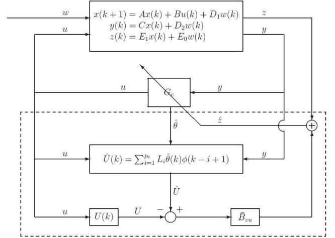
Fig. 2. Closed-loop system including adaptive control algorithm with the retrospective correction filter (dashed box) for  $p = 1$ .
