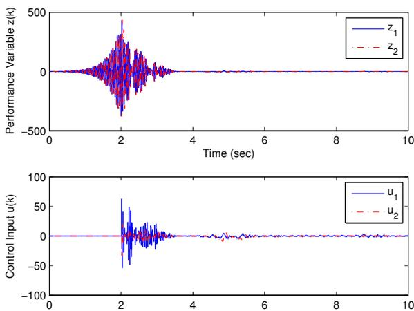
Fig. 9. Closed-loop disturbance rejection response for an unstable, nonminimum phase, two-input two-output plant. The control is turned on at  $t = 2$  sec. The controller order is  $n_c = 10$  with parameters  $p = 1$ ,  $\mu = 10$ ,  $\alpha = 1$ .
