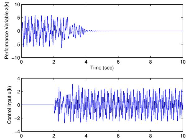
Fig. 6. Closed-loop disturbance rejection response for an IIR, stable, nonminimum phase, SISO plant. The control is turned on at  $t = 2$  sec. The controller order is  $n_c = 15$  with parameters  $p = 2$ ,  $\mu = 8$ ,  $\alpha = 25$ .
