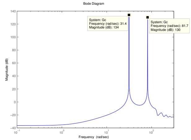
Fig. 5. Bode magnitude plot of the adaptive controller at  $t = 10$  sec. The adaptive controller places poles at the disturbance frequencies  $\nu_1 = 5$  Hz and  $\nu_2 = 13$  Hz. The controller magnitude  $|G_c(e^{j\omega T_s})|$  is plotted for  $\omega$  up to the Nyquist frequency  $\omega_{Nyq} = \frac{\pi}{T_s} = 314$  rad/sec.
