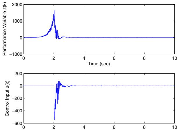
Fig. 7. Closed-loop disturbance rejection response for an unstable, minimum phase, SISO plant. The control is turned on at  $t = 2$  sec. The controller order is  $n_c = 15$  with parameters  $p = 1$ ,  $\mu = 10$ ,  $\alpha = 25$ .
