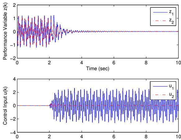
Fig. 8. Closed-loop disturbance rejection response for an IIR, stable, nonminimum phase, two-input two-output plant. The control is turned on at  $t = 2$  sec. The controller order is  $n_c = 15$  with parameters  $p = 2$ ,  $\mu = 8$ ,  $\alpha = 1$ .
