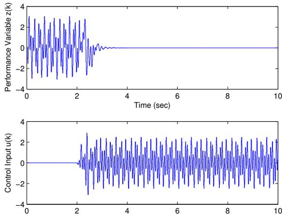
Fig. 4. Closed-loop disturbance rejection response for an IIR, stable, minimum phase, SISO plant. The control is turned on at  $t = 2$  sec. The controller order is  $n_c = 15$  with parameters  $p = 1$ ,  $\mu = 3$ ,  $\alpha = 25$ .
