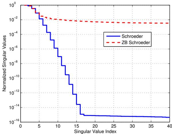
Fig. 5. Comparison of the normalized singular values of a 39<sup>th</sup> order FIR regressor matrix with a Schroeder-phased and zero-buffered Schroeder-phased signal.
