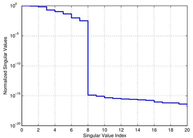
Fig. 6. Normalized singular values of the regressor matrix  $A$  given by (18) for the system (32), input (33), and order of the model  $\hat{n} = 10$ .
