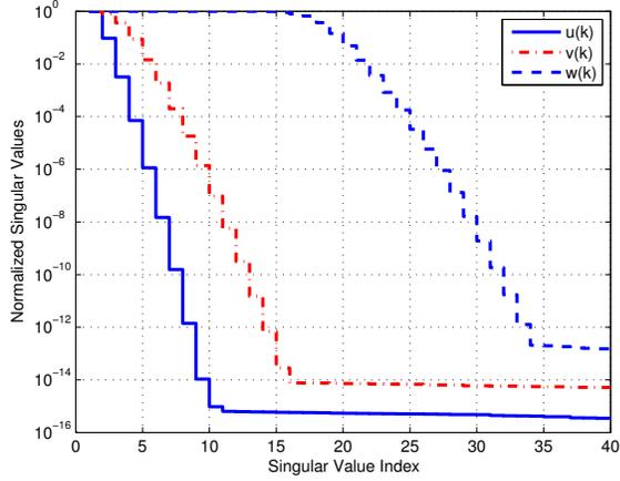
Fig. 4. Normalized singular values of the regressor matrix (4) with  $\hat{n} = 39$  and the signals (6)-(8)
