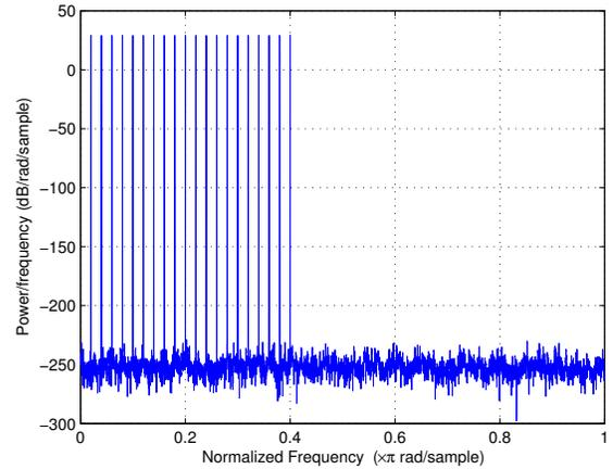
Fig. 3. Power spectral density of  $w(k)$  given by (8).
