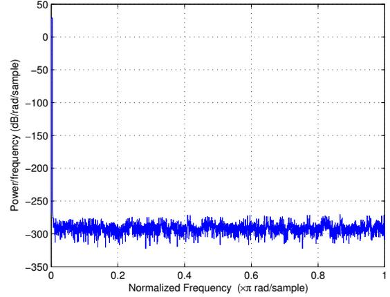
Fig. 1. Power spectral density of  $u(k)$  given by (6).
