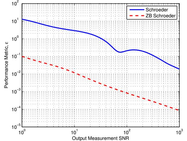
Fig. 8. Comparison of the performance metric (38) averaged over 1000 trials when the Schroeder-phased signal (35) and the zero-buffered Schroeder-phased signal (36) are used to estimate the ARX model (37) with standard least-squares.
