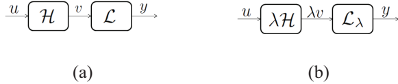
Fig. 1. (a) Block-structured Hammerstein model, where u is the input, v is the intermediate signal, y is the output, \mathcal{H} is a static nonlinearity, and \mathcal{L} is a discrete-time linear time-invariant dynamic system. (b) An equivalent scaled model, where \lambda is a scaling factor and \mathcal{L}_\lambda is a scaled-domain modification of \mathcal{L} satisfying \mathcal{L}_\lambda(\lambda v) = \mathcal{L}(v) . The scaling factor \lambda is not identifiable.
