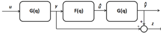
Fig. 1. Open-loop architecture for input reconstruction. In this setup, the performance z , is not used to improve the estimate \hat{u} of u .
