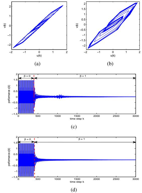
Figure 11. Example 6.4. (a) and (b) show the input nonlinearity  $\mathcal{N}(u)$  of the rate-dependent Prandtl-Ishlinskii model with (a)  $\eta = 1$ , and (b)  $\eta = 0$ . (c) and (d) show the closed-loop response to the sinusoidal command  $r(k) = 1.3 \sin(0.5\omega k) + 0.65 \sin(\omega k)$  with  $\omega = \frac{\pi}{4}$  rad/sample with the plant given by (36) and  $w(k) = 0.5 \sin(\frac{\pi}{3}k)$  when (c)  $\eta = 0$ , and (d)  $\eta = 1$ .
