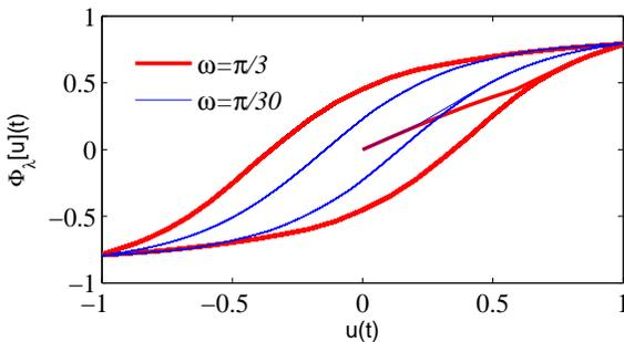
Figure 7. Example 5.3. The output of the generalized rate-dependent Prandtl-Ishlinskii model with  $\gamma(u) = 0.93 \tanh(1.85u)$ .
