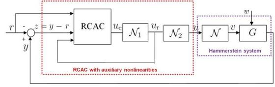
Figure 2. Hammerstein command-following problem with the RCAC adaptive controller and auxiliary nonlinearities  $\mathcal{N}_1$  and  $\mathcal{N}_2$ . The auxiliary nonlinearities are constructed based on limited knowledge of  $\mathcal{N}$ .
