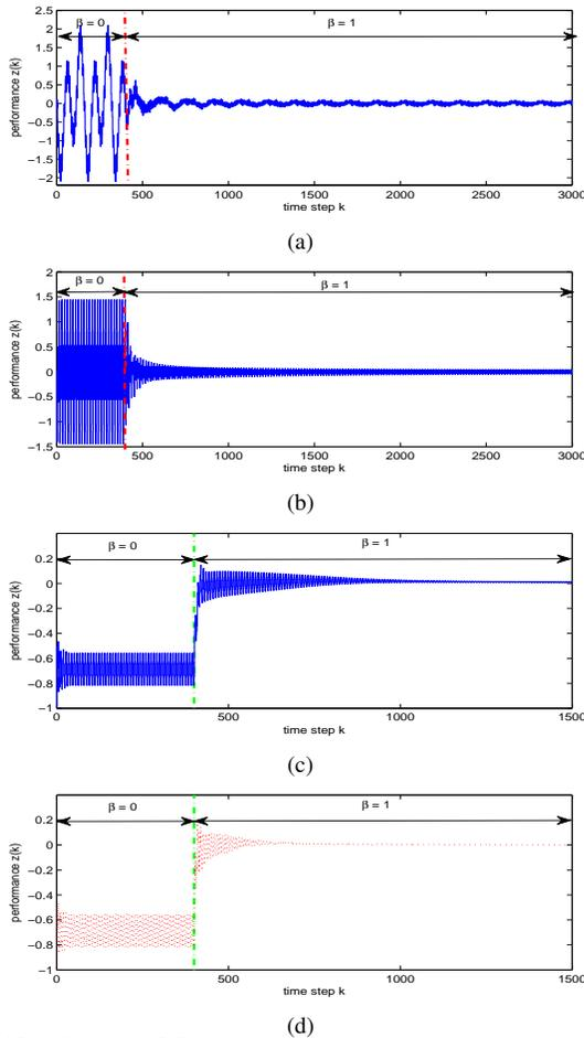
Figure 12. Example 6.5. (a) and (b) show the closed-loop response to the sinusoidal command  $r(k) = 1.3 \sin(0.5\omega k) + 0.65 \sin(\omega k)$  with  $\hat{H}_d = 2$  and  $w(k) = 0.5 \sin(\frac{\pi}{3}k)$ : (a)  $\omega = \frac{\pi}{4}$  rad/sample, and (b)  $\omega = \frac{\pi}{40}$  rad/sample. (c) shows the closed-loop response to the command signal  $r(k) = 1$  with the disturbance signal  $w(k) = 0.2 \sin(0.5\pi k)$  considering (c)  $\hat{H}_d = 2$ , and (d)  $\hat{H}_d = 1$ .
