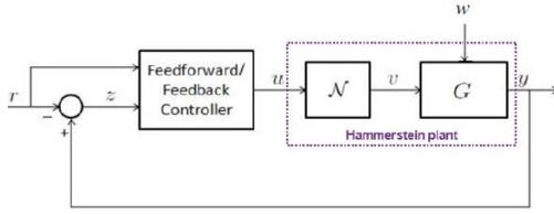
Figure 1. Adaptive command-following problem for a Hammerstein plant. We assume that measurements of  $z(k)$  are available for feedback; however, measurements of  $v = \mathcal{N}(u)$  and  $w(k)$  are not available. The feedforward path is optional.
