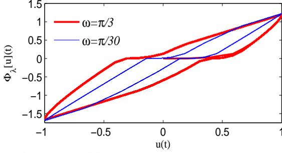
Figure 6. Example 5.3. The output of the modified rate-dependent Prandtl-Ishlinskii model.
