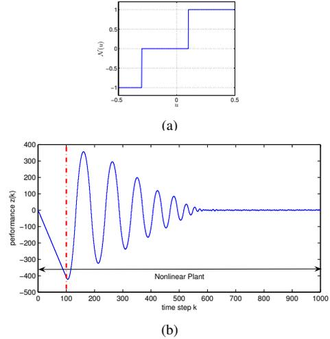
Fig. 7. Example 5.4. Closed-loop response of the plant  $G$  given by (25) with the initial condition  $x_0 = [-5.2, -1.1]^T$ . The system runs open loop for 100 time steps, and the adaptive controller is turned on at  $k=100$  with the input relay nonlinearity given by (26). The closed-loop performance  $z$  approaches  $\pm 4$  in about 500 time steps.
