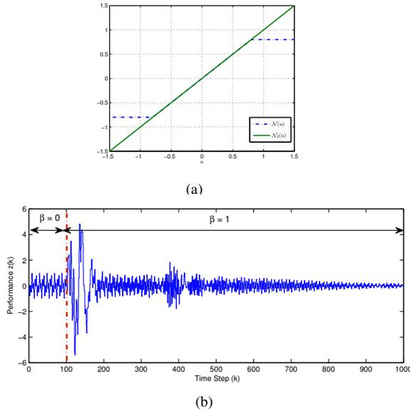
Fig. 6. Example 5.3. (a) shows the saturating input nonlinearity  $\mathcal{N}(u)$  given by (24). (b) shows the closed-loop response of the stable NMP plant  $G$  given by (22) with the two-tone sinusoidal command  $r(k) = 0.5 \sin(\theta_1 k) + 0.5 \sin(\theta_2 k)$ ,  $\theta_1 = \pi/5$  rad/sample, and  $\theta_2 = \pi/2$  rad/sample.
