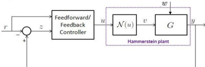
Fig. 1. Adaptive command-following problem for a Hammerstein plant. We assume that measurements of  $z(k)$  are available for feedback; however, measurements of  $v(k) = \mathcal{N}(u(k))$  and  $w(k)$  are not available. The feedforward path is optional.
