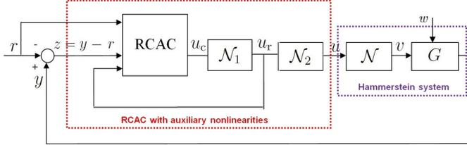
Fig. 2. Hammerstein command-following problem with the RCAC adaptive controller and auxiliary nonlinearities  $\mathcal{N}_1$  and  $\mathcal{N}_2$ .
