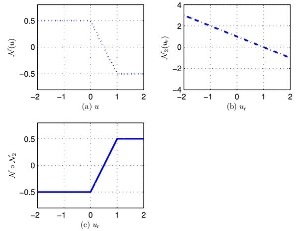
Fig. 3. (a) Input nonlinearity  $\mathcal{N}(u) = -\text{sat}_{0.5,0.5}(u - 0.5)$ . (b) Auxiliary nonlinearity  $\mathcal{N}_2(u_r) = -u_r + 1$  for  $u_r \in [-2, 2]$ . (c) Composite nonlinearity  $\mathcal{N} \circ \mathcal{N}_2$ . Note that  $\mathcal{N} \circ \mathcal{N}_2$  is nondecreasing and  $\mathcal{R}(\mathcal{N} \circ \mathcal{N}_2) = \mathcal{R}(\mathcal{N}) = [-0.5, 0.5]$ .
