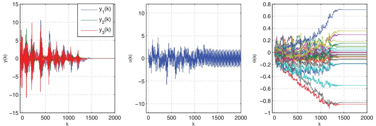
Figure 4. Example 4.3: Matched disturbance rejection for the minimum phase,  $3 \times 1$  tall plant (40) and (41). The controller  $\Theta$  converges,  $u$  is bounded, and  $y$  asymptotically approaches zero. RCAC cancels the matched sinusoidal disturbance from three outputs using only one actuator.
