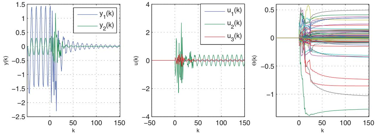
Figure 2. Example 4.1: unmatched disturbance rejection for the minimum-phase,  $2 \times 3$  wide plant (38) and (39). The performance output  $y$  approaches zero, the control signal  $u$  is bounded, and the controller  $\Theta$  converges.
