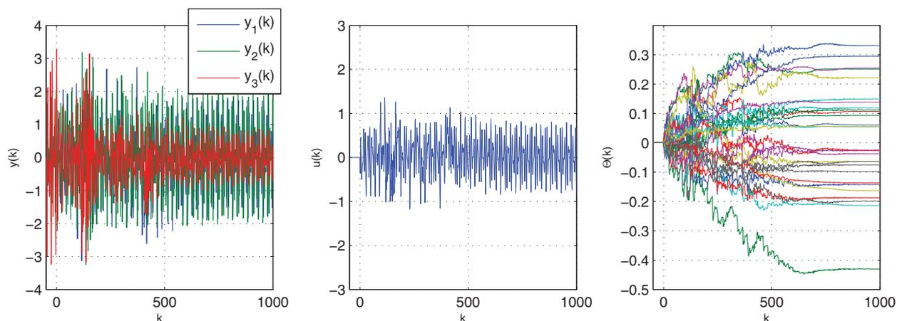
Figure 5. Example 4.5: Unmatched disturbance rejection for the minimum-phase,  $3 \times 1$  tall plant of Example 4.3 with  $D_1 = [0 \ 1 \ 0]^T$ . The controller  $\Theta$  converges, and the signals  $u$  and  $y$  are bounded. The performance output  $y$  does not converge to zero due to the infeasibility of the unmatched disturbance rejection problem in the tall case.
