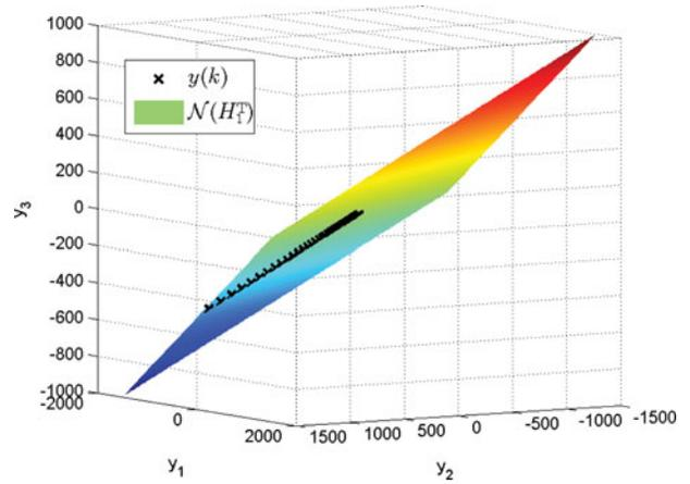
Figure 10. This figure illustrates the phase portrait for  $k \in [100, 200]$  of the unbounded performance output  $y$  for Example 4.5 shown in Figure 6. Since the output-subspace zeros of  $G_{yu}$  are NMP, the unbounded output  $y$  grows without bound on the surface  $\mathcal{N}(H_1^T)$ . Since  $y$  is contained in  $\mathcal{N}(H_1^T)$ , the controller  $\Theta$  in Figure 6 converges despite the fact that  $y$  is unbounded.
