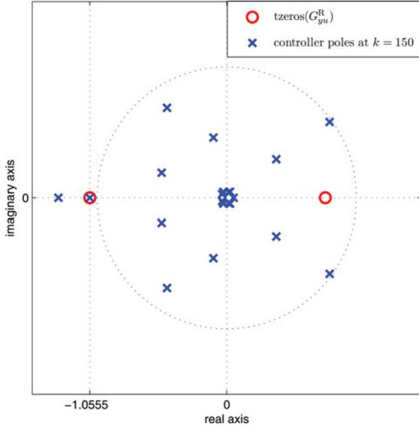
Figure 8. This figure illustrates the input-subspace zeros of the plant in Example 4.2 along with the poles of the adaptive controller at  $k = 150$ , whose time evolution is shown in Figure 3. The adaptive controller places a pole near the NMP input-subspace zero of  $G_{yu}$ , which is located at  $-1.0555$ . This unstable pole-zero cancellation is the cause of the unbounded control input shown in Figure 3. Note that the NMP input-subspace zero is not a transmission zero of  $G_{yu}$ .
