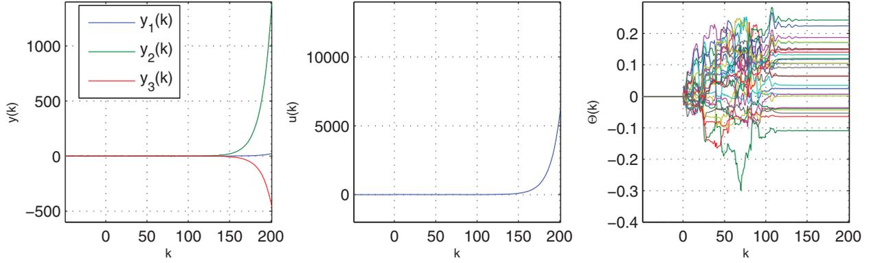
Figure 6. Example 4.5: Unmatched disturbance rejection for the  $3 \times 1$  tall plant of Example 4.4 except that  $C_{(1,2)} = 0.6$ . Although  $G_{yu}$  is minimum phase, the signals  $u$  and  $y$  grow without bound. The controller  $\Theta$  converges.
