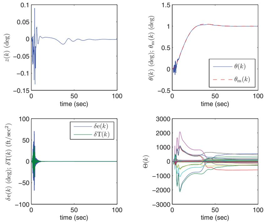
Figure 16. Boeing 747 longitudinal dynamics: We apply RCAC without  $\eta$ -modification. Although the pitch angle follows the output of the reference model, the elevator deflection and thrust excursion oscillate during the transient with peak magnitudes 71 deg and 36 ft/sec<sup>2</sup>, respectively. The control inputs are not within practical saturation limits.
