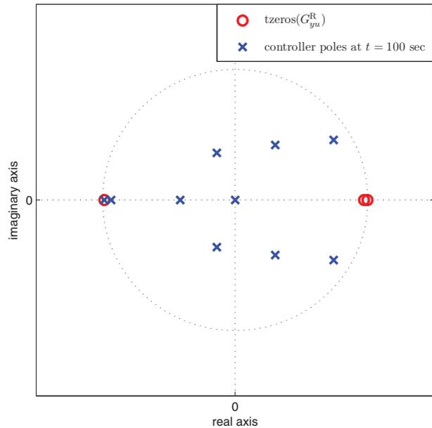
Figure 17. This figure illustrates the input-subspace zeros of the Boeing 747 longitudinal dynamics along with the poles of the adaptive controller at  $t = 100$  sec. The adaptive controller places a pole near the input-subspace zero  $-0.9857$ . This pole-zero cancellation near the unit circle causes large transients in the elevator deflection and thrust excursion, as illustrated in Figure 16.
