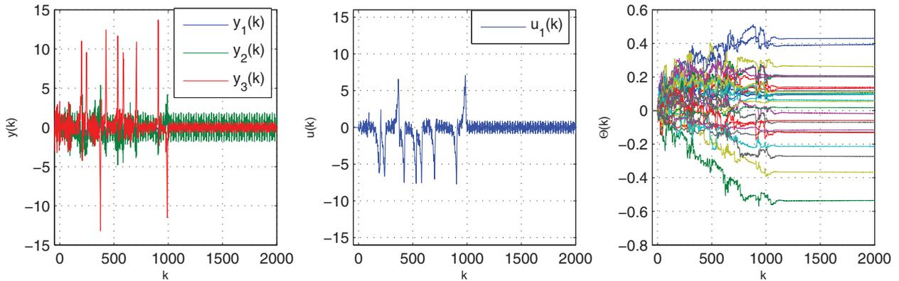
Figure 15. Example 4.5, RCAC with  $\eta$ -modification: We consider the same plant and disturbance as in Example 4.5, and apply the instantaneous update law with  $\eta$ -modification. We use  $n_c = 7$ ,  $\mu = 20$ ,  $\eta_0 = 0$ , and  $\eta_1 = 0.01$ . Despite the unmodelled NMP output-subspace zero,  $\Theta$  converges, and  $u$  and  $y$  are bounded.
