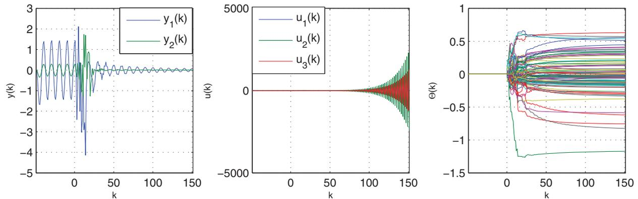
Figure 3. Example 4.2: unmatched disturbance rejection for the  $2 \times 3$  wide plant (38) and (39) except that  $B_{(1,1)} = -1.8$ . Although  $G_{yu}$  is minimum phase, the control signal  $u$  grows without bound, while the performance output  $y$  approaches zero. The controller  $\Theta$  converges.
