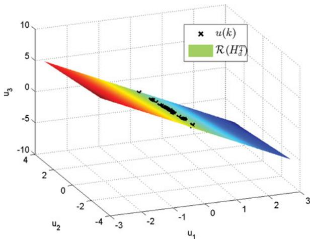
Figure 9. This figure illustrates the phase portrait of the bounded control input  $u$  for Example 4.1 shown in Figure 2. For all  $k \geq 1$ ,  $u(k)$  is contained in the subspace  $\mathcal{R}(H_d^T)$ , which is the coloured plane in this figure. The control input is bounded due to the fact that the input-subspace zeros of  $G_{yu}$  are minimum phase.
