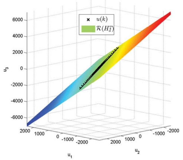
Figure 7. This figure illustrates the phase portrait of the unbounded control input  $u$  for Example 4.2 shown in Figure 6. For all  $k \geq 1$ ,  $u(k)$  is contained in the subspace  $\mathcal{R}(H_1^T)$ , which is the coloured plane in this figure. The control input is unbounded due to the fact that the input-subspace zeros of  $G_{yu}$  are NMP.
