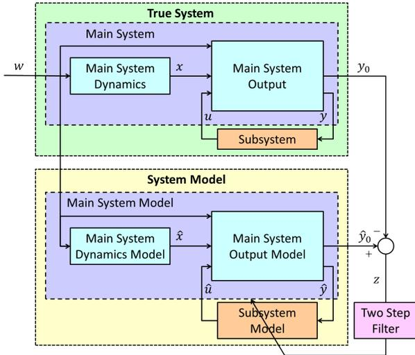
Fig. 1. The architecture for the Two Step Filter.
