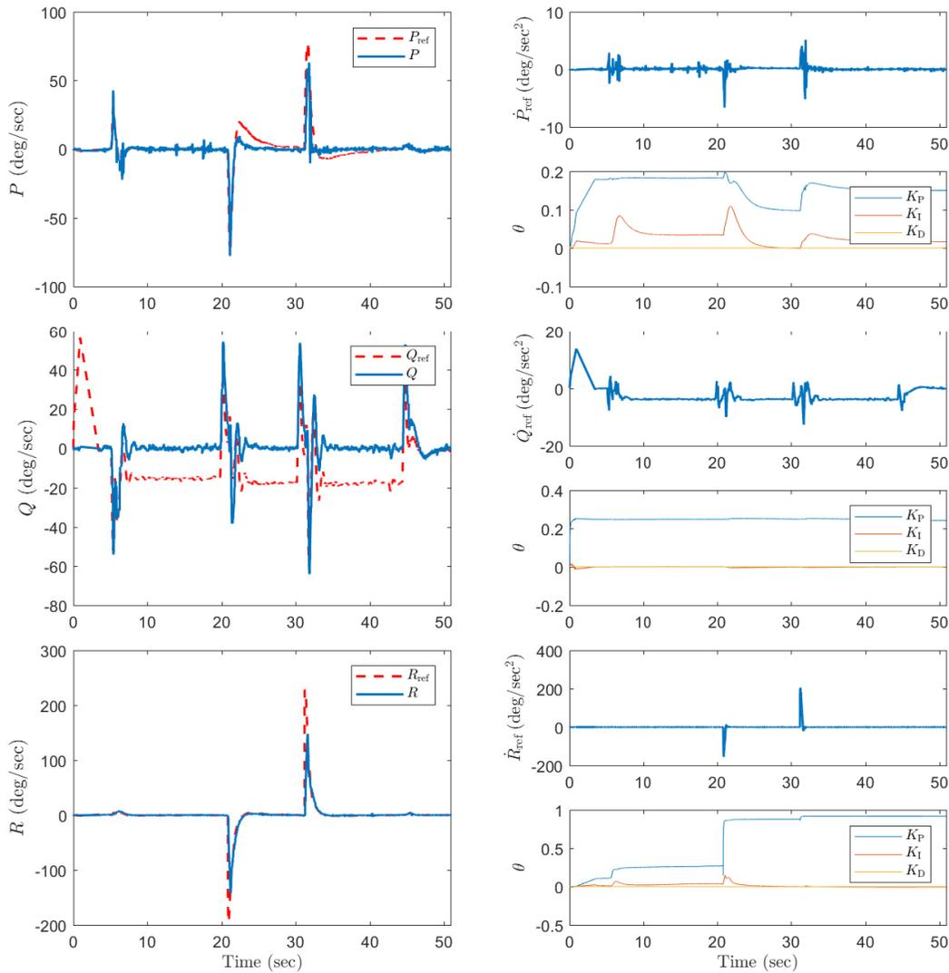
Figure 5. Performance of the quadcopter inner-loop RC-PID for angular-velocity commands. The controller coefficients  $\theta$  converge for each RC-PID controller. At  $t = 50.8$  sec, the command-following errors in the angular-velocity components  $P$ ,  $Q$ , and  $R$  are  $0.3$  deg/sec,  $1$  deg/sec, and  $-0.2$  deg/sec, respectively.
