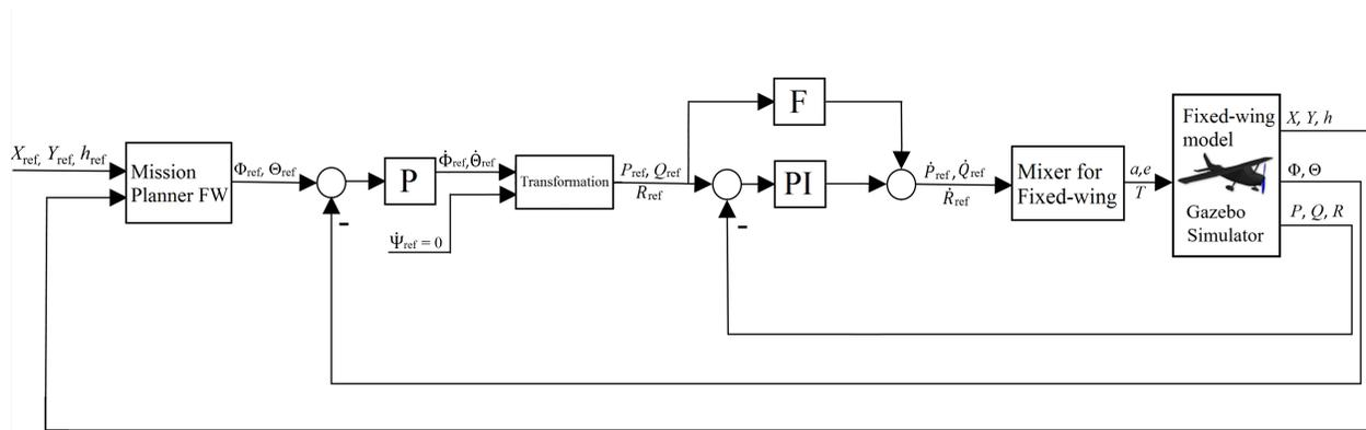
Figure 7. Interface of the PX4 flight stack with Gazebo for a fixed-wing aircraft. The middle loop consists of two P controllers to follow the Euler-angle commands  $(\Phi_{ref}, \Theta_{ref})$ , whereas the inner loop consists of three feedforward-augmented-PI controllers to follow the angular-velocity commands  $(P_{ref}, Q_{ref}, R_{ref})$ .
