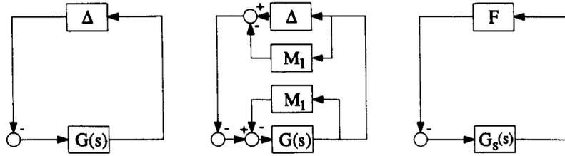
Fig. 2. Loop-shifting transformation.
