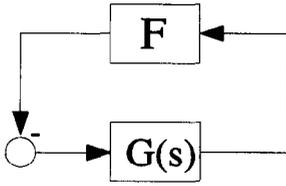
Fig. 1. Interconnection of transfer function  $G(s)$  with real uncertain matrix  $F$ .
