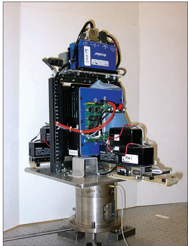
Figure 2. Photograph of the air spindle testbed. A pair of proof mass actuators are mounted on a rectangular platform in accordance with the arrangement shown in Figure 1.
