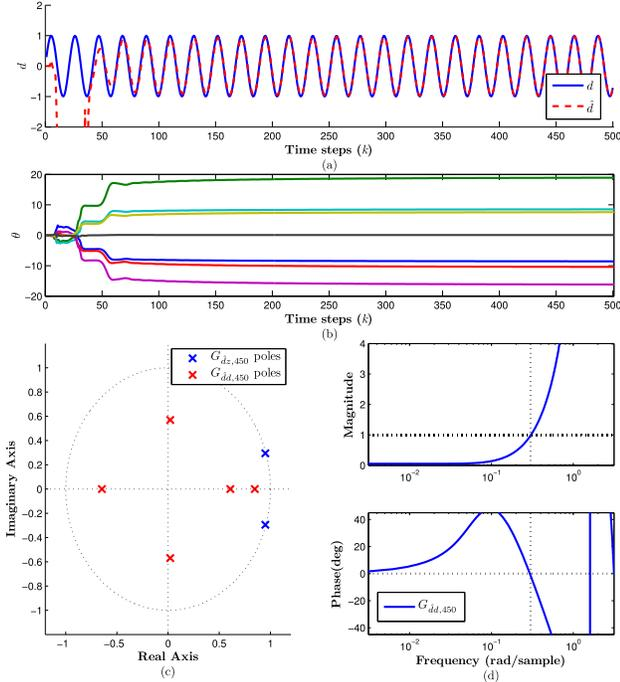
Fig. 4. RCIE for the NMP system (71). (a) After the initial transient,  $\hat{d}$  follows  $d$ . (b) Estimator coefficients  $\theta$  converge in about 450 steps. (c) Poles of  $G_{\hat{d}z,450}$  at  $0.95 \pm 0.29j$  show that RCIE builds an internal model of  $d$  in  $G_{\hat{d}z}$ . The poles of  $G_{\hat{d}d,450}$  are inside the open unit disk. (d)  $G_{\hat{d}d}$  has magnitude 1 and phase  $0^\circ$  at the unknown input frequency 0.3 rad/s.
