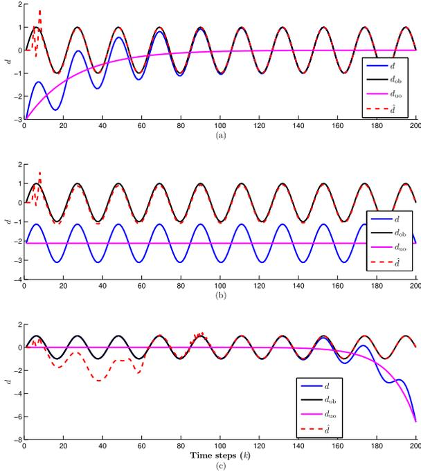
Fig. 6. Effect of the unobservable input subspace on the estimate of the unknown input using RCIE for the system (76). (a)  $\hat{d}$  converges to  $d_{ob}$ , and  $d_{uo} = d - d_{ob}$  converges to zero. (b)  $\hat{d}$  converges to  $d_{ob}$ , and  $d_{uo} = d - d_{ob}$  is a nonzero constant. (c)  $\hat{d}$  converges to  $d_{ob}$ , and  $d_{uo} = d - d_{ob}$  diverges.
