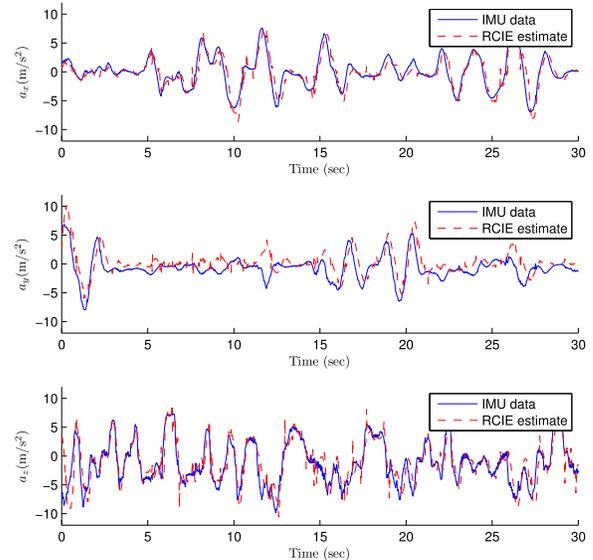
Fig. 11. Estimation of the inertial acceleration of the quadrotor relative to  $O_E$  with respect to  $F_B$  using position and attitude measurements. RCIE estimates are compared with the IMU acceleration measurements with gravity correction.
