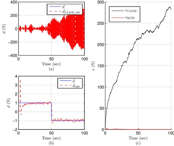
Fig. 9. Estimation of an unknown multistep input for the mass-spring system (79) with  $c_1 = c_2 = 0$ . (a) ULISE estimate. (b) RCIE estimate. (c) Error in the input estimate. The RCIE error is close to zero, whereas the ULISE error diverges.
