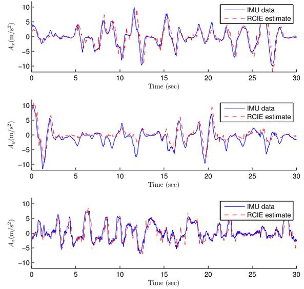
Fig. 10. Estimation of the inertial acceleration of the quadrotor relative to  $O_E$  with respect to  $F_E$  using position measurements. RCIE estimates are compared with the IMU acceleration measurements transformed to  $F_E$  and corrected to compensate for gravity offset.
