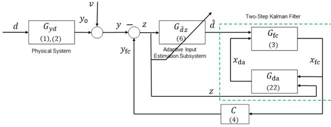
Fig. 1. Block diagram of RCIE. The two-step Kalman filter consists of the forecast subsystem  $G_{fc}$  and the data-assimilation subsystem  $G_{da}$ . The innovation  $z$  and the output  $\hat{d}$  of the input-estimation subsystem  $G_{\hat{d}z}$  are the inputs of the two-step Kalman filter.
