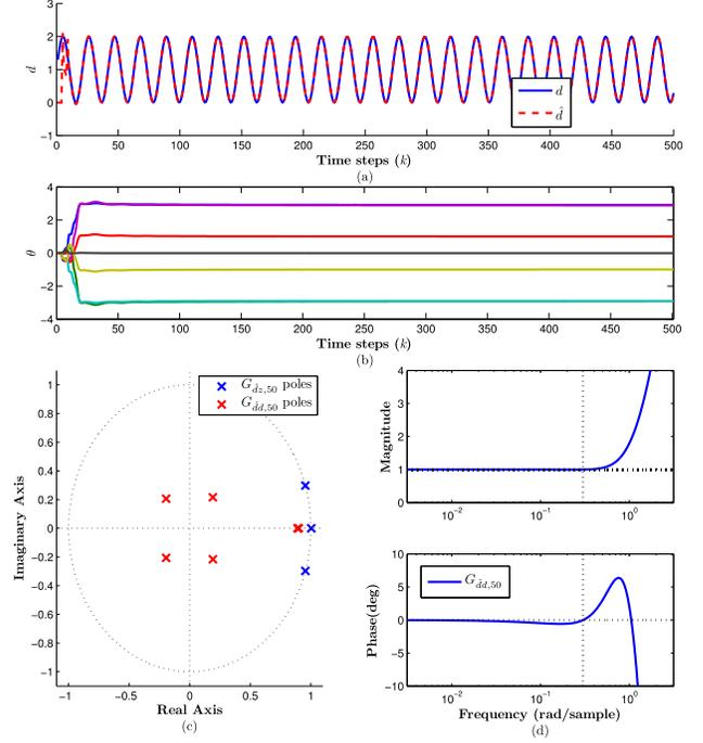
Fig. 2. RCIE for the MP system (67). (a) After the initial transient,  $\hat{d}$  follows  $d$ . (b) Estimator coefficients  $\theta$  converge in about 50 steps. (c) Poles of  $G_{\hat{d}z,50}$  at  $1.004$  and  $0.95 \pm 0.29j$  show that RCIE builds an internal model of  $d$  in  $G_{\hat{d}z,50}$ . The poles of  $G_{\hat{d}d,50}$  are inside the open unit disk. (d)  $G_{\hat{d}d,50}$  has magnitude 1 and phase  $0^\circ$  at both dc and the unknown input frequency 0.3 rad/s.
