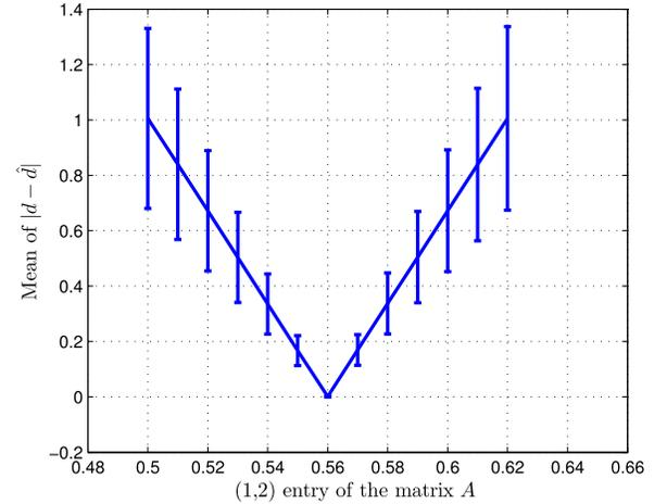
Fig. 3. Robustness of RCIE to model error for the system (67). The (1, 2) entry of  $A$  is varied while keeping the matrices  $G, C$ , and RCIE parameters constant. Note that the mean and standard deviation of the error increase linearly as the (1, 2) entry of  $A$  varies from its true value 0.56.
