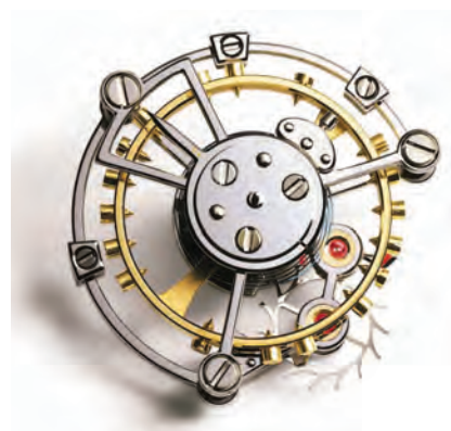
FIGURE 3 Breguet tourbillon. An offset of the center of mass of the balance wheel from its axis of rotation causes the time-keeping rate of the watch to vary as the tilt angle of the watch changes. By continually rotating the entire balance wheel, hairspring, and escape-wheel assembly about the balance wheel's axis of rotation, this rate bias is averaged, and thus the timekeeping rate becomes independent of the tilt angle. (Image courtesy of Montres Breguet SA.)
