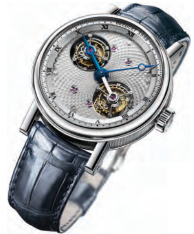
FIGURE 5 The Breguet Classique Grande Complication wristwatch, in platinum with sapphire crystal, features twin rotating tourbillons. The tourbillons are coupled by means of differential gears and mounted on a rotating center plate, which completes one revolution every 12 hours. The differential conveys the tourbillons’ mean rate to the hands of the watch. The rate of the watch is thus the mean rate of the two tourbillons. (Image courtesy of Montres Breguet SA.)
