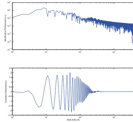
Fig. 11. Performance comparison. The upper plot shows the identification performance  $e_z$ . The lower plot shows the controller performance  $z$ .
