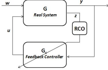
Fig. 1. Disturbance rejection and command following architecture.
