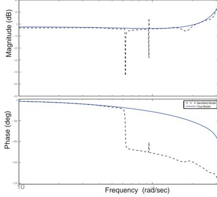
Fig. 5. Frequency response comparison of the true system  $G_{zu}$  and the estimated system  $\hat{G}_{zu}(k)$ , where  $k = 1000$ .
