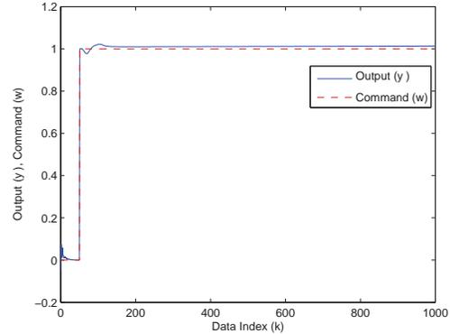
Fig. 8. Plant output for command following. The goal is to have the system trajectory follow a step command.
