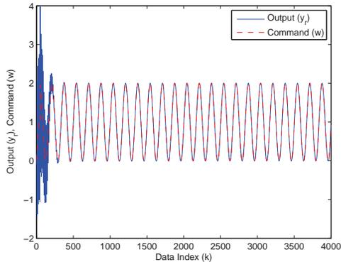
Fig. 10. Plant output for command following. The goal is to have the system trajectory follow a step command and a periodic signal, while also rejecting a periodic disturbance.
