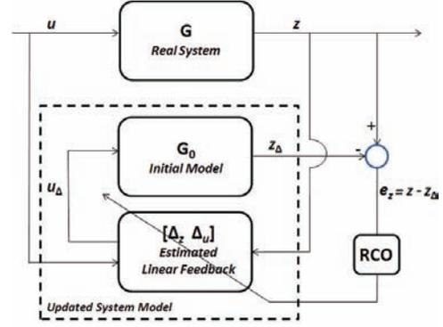
Fig. 2. Retrospective-cost model identification. The identified model resides in the dashed box. The diagonal arrow represents data-driven adaptation.
