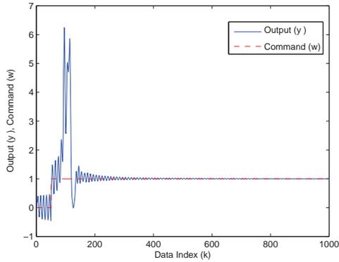
Fig. 9. Plant output for command following. The goal is to have the system trajectory follow a step command, while also rejecting a periodic disturbance.
