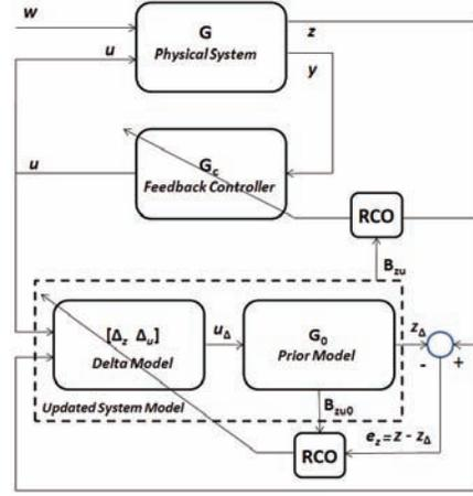
Fig. 3. The hybrid architecture is created by combining the direct retrospective-cost adaptive control and retrospective-cost model identification architectures.
