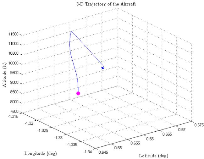
Fig. 2. Trajectory of the aircraft as it maneuvers towards the asymptotically stable trim state. The initial trim is denoted by a magenta dot.
