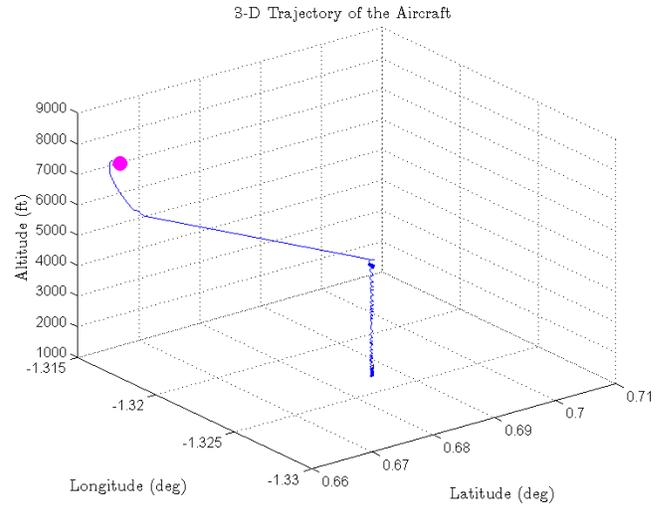
Fig. 4. Trajectory of the aircraft as it maneuvers towards the trim state that is not asymptotically stable. The initial trim is denoted by a magenta dot.
