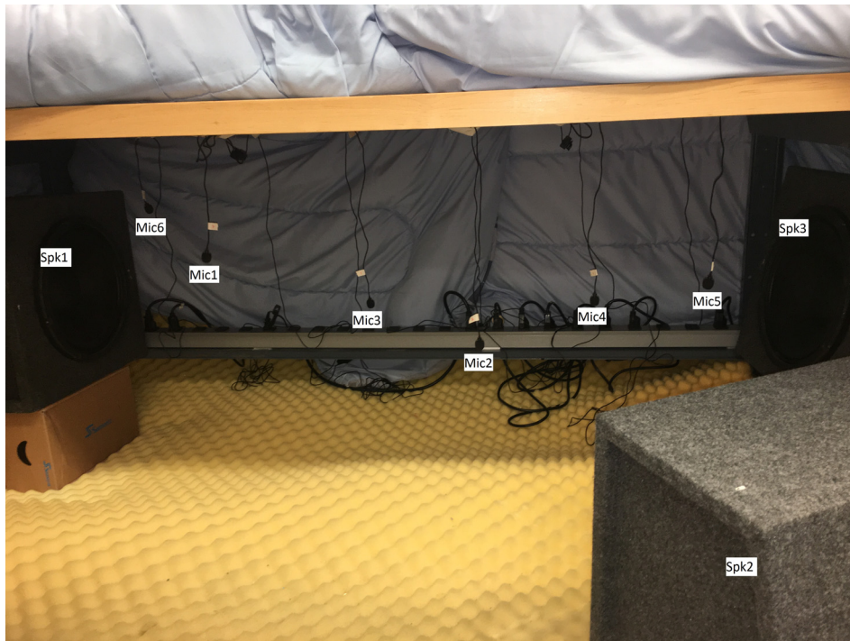
Fig. 1 Experimental setup. The setup consists of an acoustic space with three speakers Spk1, Spk2, and Spk3 and six microphones Mic1, ..., Mic6. Each speaker is an actuator, and each microphone is a sensor that measures the acoustic response at its location.
