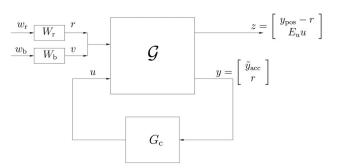
Fig. 1 Standard problem for designing a position-tracking controller  $G_c$  that uses biased acceleration measurements. To facilitate controller synthesis using LQG, the backward-path controller  $G_{\rm bp}$  that is used to reject the sensor bias is included in the Plant  $\mathcal{G}$ .
