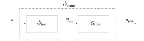
Fig. 3 Construction of the compliance  $\hat{G}_{comp}$  by cascading a double integrator with the identified inertance
