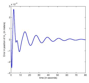
Fig. 5 Error between the actual position of  $m_1$  and the output  $y_{\text{pos},1}$  of the identified compliance model when  $u_1$  is an impulse and  $u_2=0$ . For position-tracking controller synthesis, the identified compliance is used.
