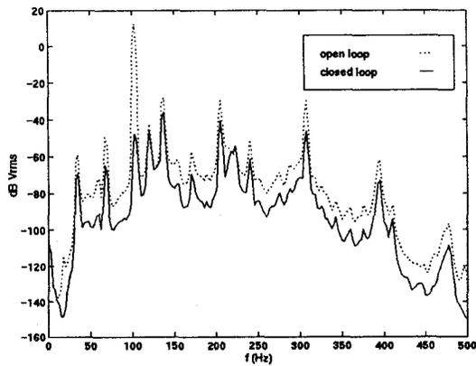
Figure 7: Performance Spectrum  $z$  - ARMARKOV with fan
