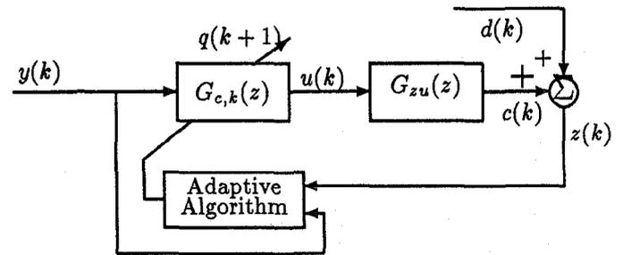
Figure 2: Block Diagram of Adaptive Control Law and Error Path
