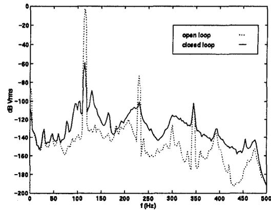
Figure 5: Performance Spectrum  $z$  - FUREC with a single tone
