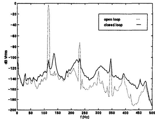
Figure 6: Performance Spectrum  $z$  - ARMARKOV with a single tone
