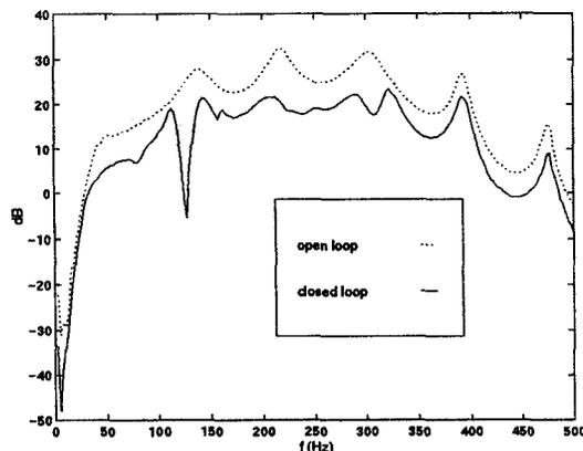
Figure 8:  $G_{zw}$  - ARMARKOV with white noise
