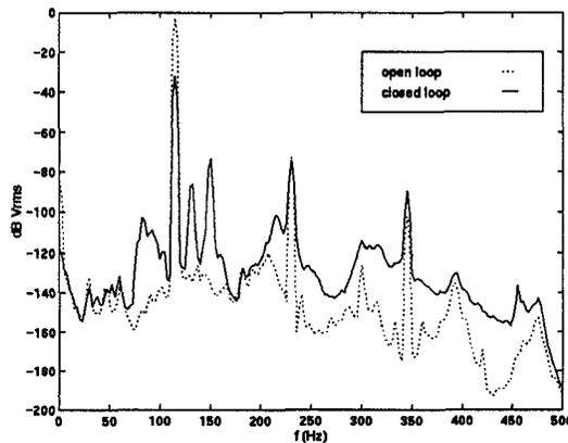
Figure 4: Performance Spectrum  $z$  - FXLMS with a single tone
