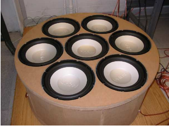
Figure 4: Control actuator configuration. The 7-speaker arrangement provides acoustic actuation of the membrane displacement.
