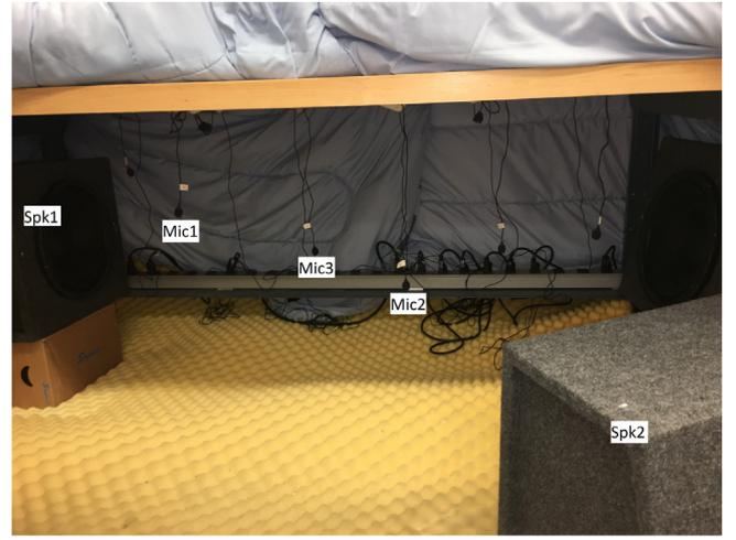
**Fig. 8.** Acoustic experiment setup. Two speakers and three microphones are used in the experiment to excite the three-dimensional acoustic space and measure its response.
