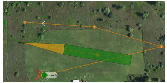
Fig. 5. Waypoints used to construct the flight trajectory in simulation experiments.
