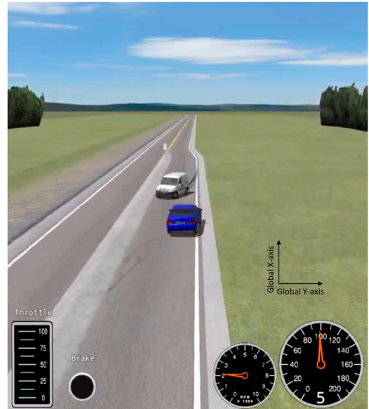
Figure 12. Collision-avoidance scenario in CarSim. In this scenario, the oncoming vehicle (the white van) enters the opposite lane, and the host vehicle (the blue van) performs an evasive maneuver to avoid a collision.
